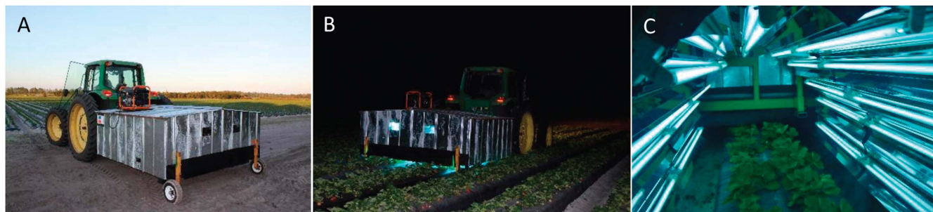
Fig. 2. UV-C tractor-drawn wheeled equipment for UV treatments. A , Side view of the UV-C tractor-drawn unit. B , Unit during nighttime field operation. C , View of interior showing the dense reflectorized hemicylindrical array of germicidal UV-C lamps.
